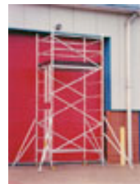
(Above) Mobile Scaffold
